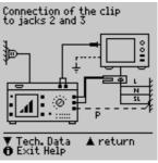
P: potential lead for 4-wire measurement
