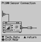
Temperature can be measured within a range of -200 °C to +850 °C with a Pt100 or Pt1000 sensor (default setting) connected to the PE (1) and N (2) jacks.
