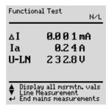
The test socket can be rendered voltage-free with the key (14), or the function test can be ended with the  $\checkmark$  key (12).
