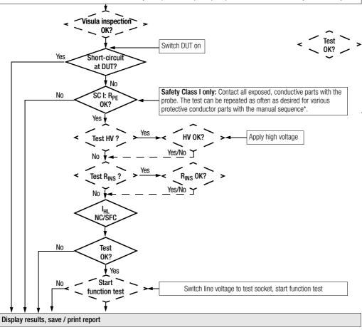
Framed with dashed line: The test is only run if it has been activated in the **Setup** menu under **Sequence...**
