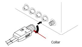
Note: When disconnecting the output connector and the measuring instrument, be sure to release the lock by rotating the collar in the opposite direction of the arrow as shown in the figure above before pulling off the connector. Forcibly pulling the connector without releasing the lock or pulling on the cable can damage the terminator.
