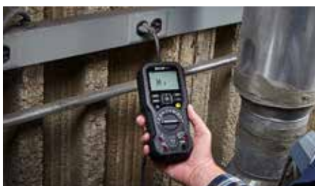
Check if voltage is present with the built-in Non-Contact Voltage detector (NCV)
